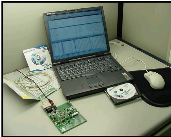
The ADuC8xx QuickStart Development System
