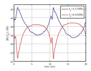
Fig. 1: Time evolution of the amplitude response along the mains cycle at two frequencies.
