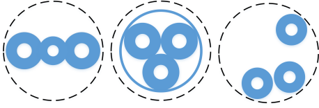
Fig. 4. Cross section of typical cables used in in-home power grids: multipolar ribbon (left), multipolar symmetric (center) and monopolar (right). The dashed circumference represents the ribbed plastic tube where in-home cabling is usually enclosed in.
