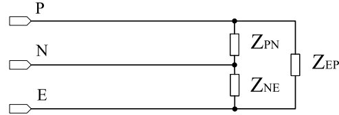
Fig. 6. Lumped element model for in-home grid ends. Each Z_{ij} impedance is modeled as a series connection of parallel RLC circuits.
