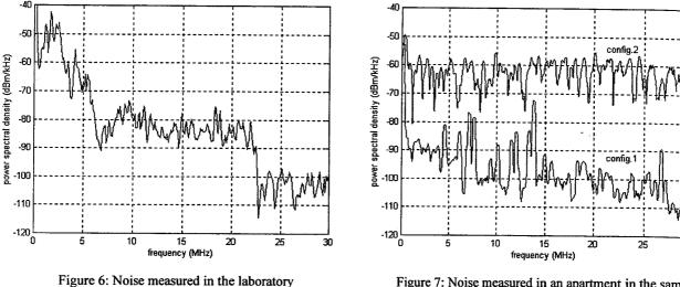
Figure 7: Noise measured in an apartment in the same situation, but in config.2 additional electrical appliances were turn on.
