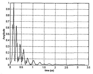
Figure 1: Impulse response of modelled channel (normalised).
