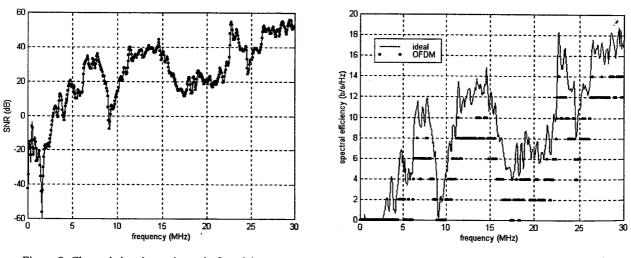
Figure 8: Channel signal to noise ratio for a laboratory measurement.
