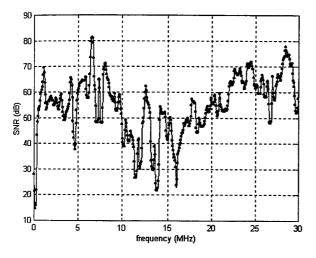
Figure 10: Channel signal to noise ratio for an apartment measurement. Best conditions of load
