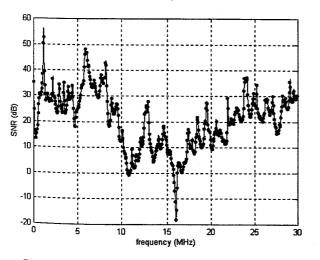
Figure 12: Channel signal to noise ratio for an apartment measurement. Worst conditions of load.
